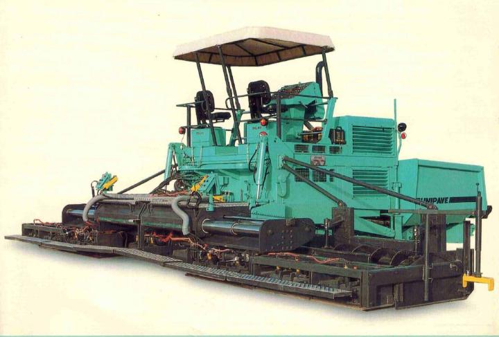
AUTOPAVE 175 is a crawler mounted Paver designed for paving width up to 9 meters. Two hydraulic circuits, synchronized electronically, drive the crawler chain, which can be easily controlled from operating panel by simple rotary buttons. Two variable
