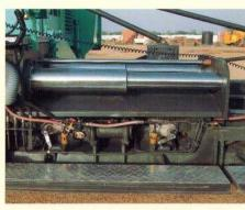
Screed model HX5590 has a basic width of 3 meters and can be hydraulically extended up to 5.5 meters. The mobile part of the screed moves on two heavy telescopic cylindrical guides. These guides are hard chrome plated for wear resistance. The Screed can be further extended up to 9 meters by bolt on extension screed plates for paving
